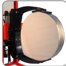
Opening the gripping arms by mistake is not possible. Clear indication whether the clamping force is sufficient for lifting/rotating.
